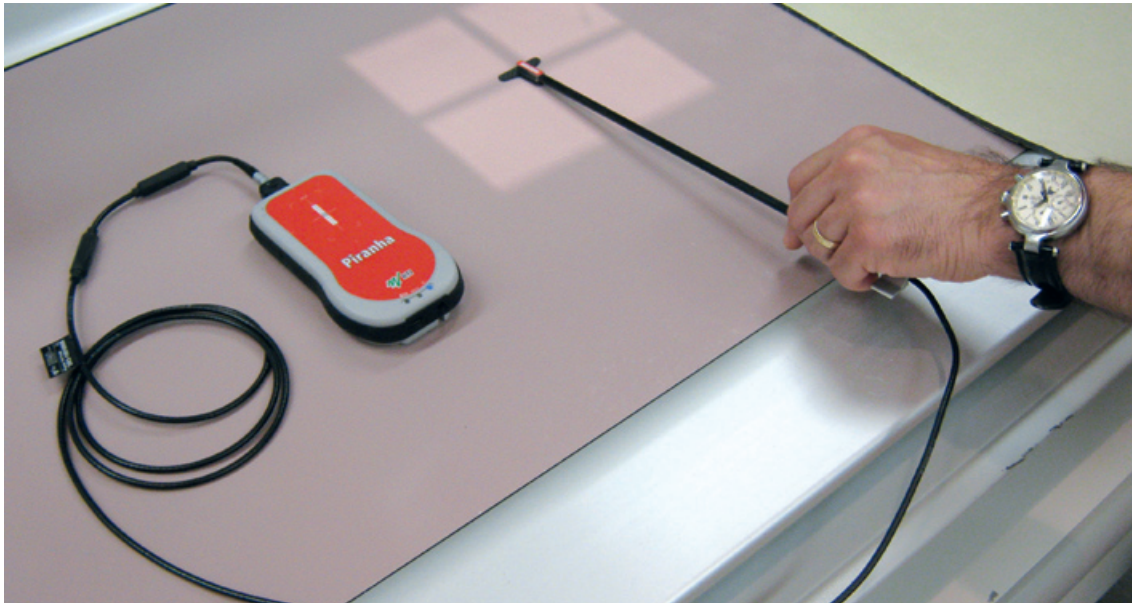
The T20 is connected to a 280 mm carbon fiber rod, allowing for measurements on an II as large as 45 x 45 cm.
